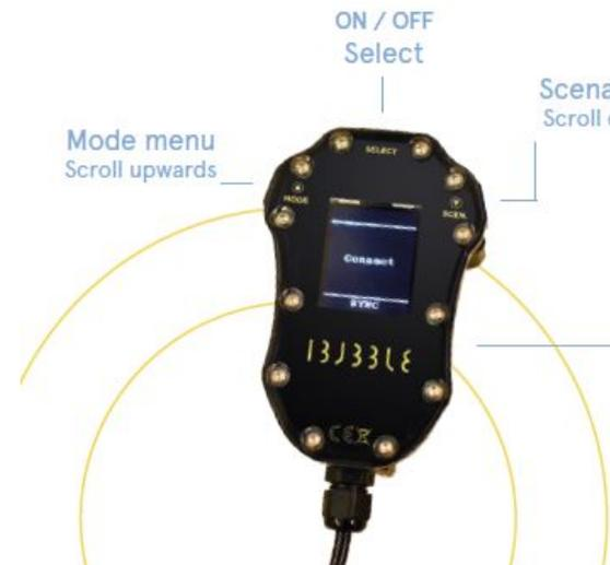
The remote control allows you to control the drone when immersed. The buttons are used to browse the different menus.
