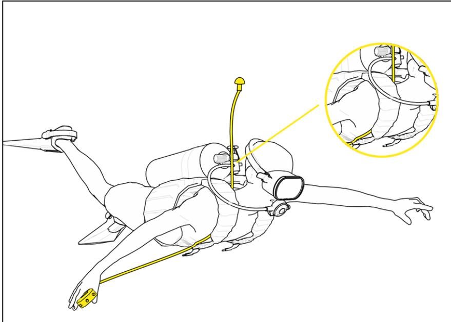
The remote is equipped with a cable at the end of which is an acoustic transmitter. This transmitter is used by iBubble to position itself. It must remain visible to the drone at all times. Avoid positioning it where it would be hidden.
